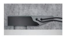
► The trimless installation in cast concrete ceilings can be realised using specially developed cast-in housings. The use of a variable core element means this is also possible with bare concrete ceilings.
