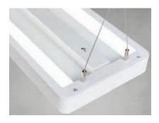
Luminaire with direct/indirect emisson, equipped with LED-Arrays in COB (Chipon-board) technology. Above 100 lm/W and outstanding long durability. L90/B10 -  $50000\,hrs$ , 3 Step MacAdam, CRI > 84.
