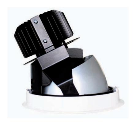
These LED spotlights can fulfil completely different tasks – ranging from glare-free general lighting to variable, point-precise light accents. The spotlights can be rotated through 350° and tilted between 30° and 50°. The product range was designed as flexible lighting tools and features a uniform luminaire design with three variants, two sizes and five light distribution characteristics.
